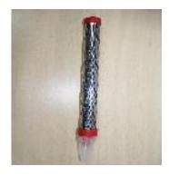
The use of trap is relatively a new method of detecting, trapping insects in stored grains. The basic components of a TNAU probe trap consists of three important parts: A main tube, insect trapping tube and a detachable cone at the bottom. Equispaced perforations of 2 mm diameter are made in the main tube.
